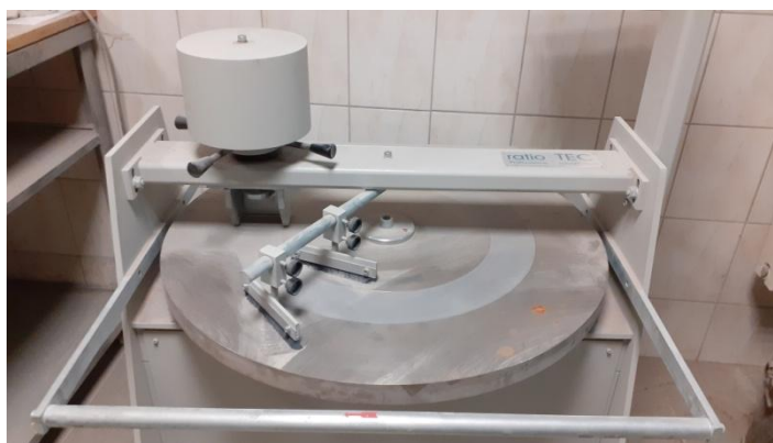
Fig.2. Boehme wheel for determining grindability of stone materials
