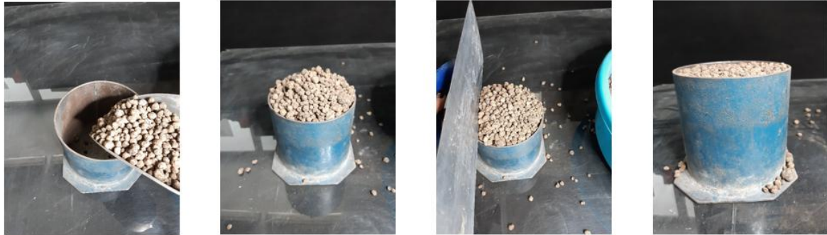
Fig2. The course of the examination of the bulk density
