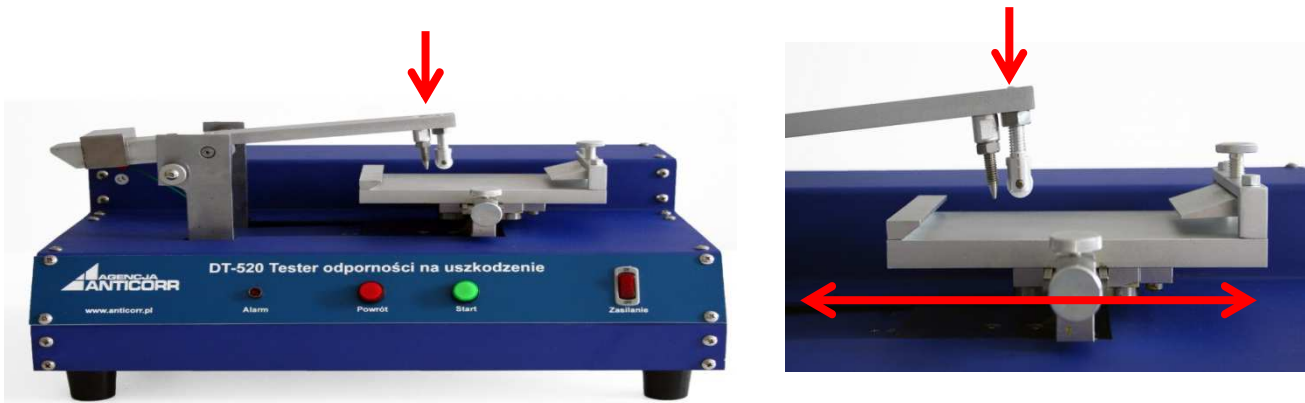
Fig. 3. Testing scratch resistance of paint coatings using Clemen apparatus (Anyicor) [photo source: https://anticorr.pl/clemen-test,p,354,863.html ]
